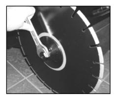
Figure 12: Tightening Nut
